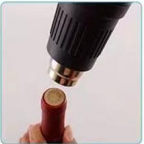
5.Blow the cap from top to bottom with a hot air gun
